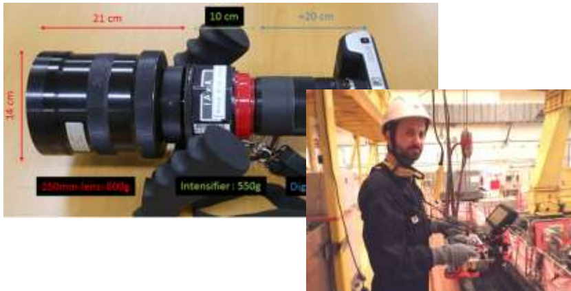
ICVD in a configuration with 250mm lens and an example of digital back
