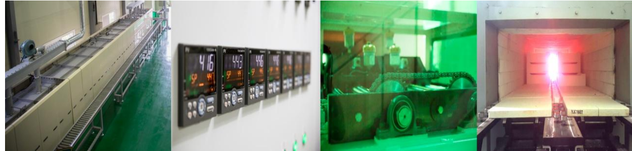
Temperature-varying calcination at 1,000°C for 24 hours by patented technology of our company
