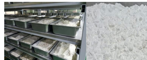
Production of highly purified calcium by nine day maturation of calcinated coral calcium
