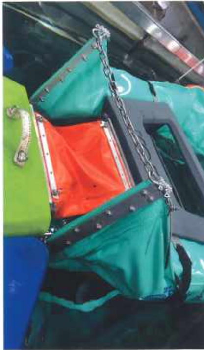
spilled oil collecting system (completion of assembly)
