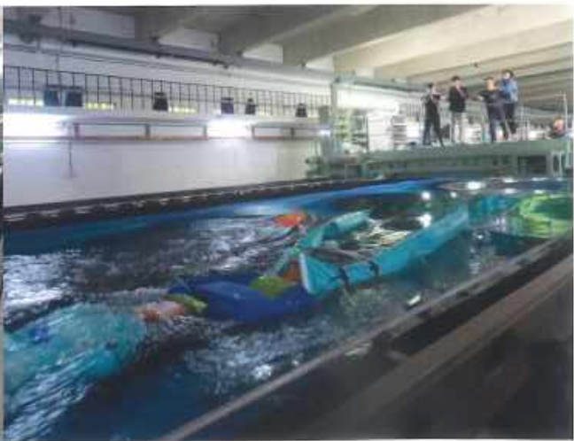
Automatic spilled oil collecting device for large area
