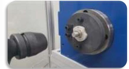
**Junker test (DIN65151) – Supported from Lim Jin ST**
